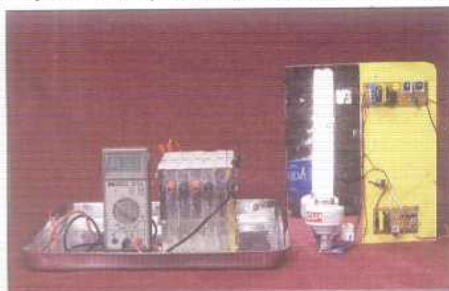
28W Direct Borohydride Fuel Cell (DBFC)
