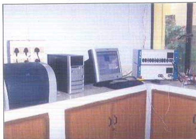
A prototype fuel cell assembled at this unit is being evaluated using Multistat Potentiostat / Galvanostat with frequency response analyzer (Solatron).
